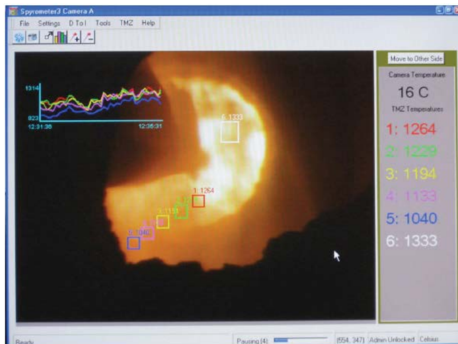
Figure 6.2-1 – Screenshot from a Mirion Pyrometer Camera (M555/M215)
